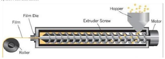
In hot melt extrusion method, firstly the drug is mixed with carriers in solid form. Then the extruder having heaters melts the mixture and finally the melt is shaped in to films by the dies. There are certain benefits of hot melt extrusion which includes-
