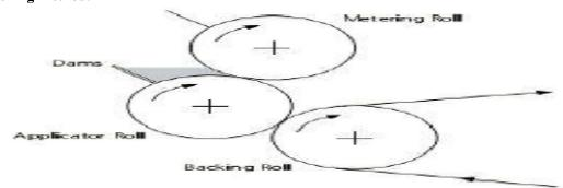
In rolling method, a solution or suspension containing drug is rolled on a carrier. The solvent is mainly water and mixture of water and alcohol. The film is dried on the rollers and cutted in to desired shapes and sizes. Other ingredients including active agent are dissolved in small portion of aqueous solvent using high shear processor. Water soluble hydrocolloids dissolved in water to form homogenous viscous solution.
