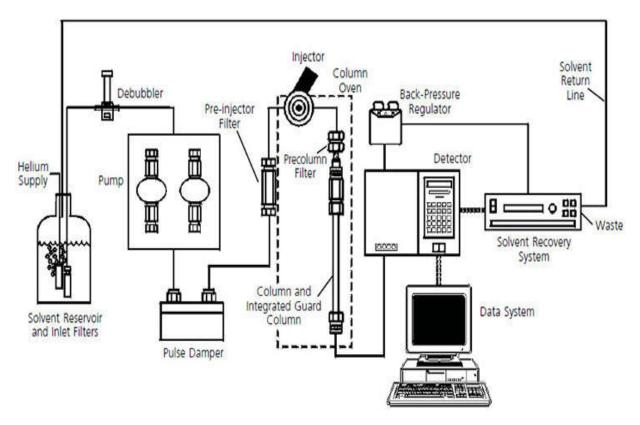
The instrumentation of UPLC includes- sample injection, UPLC columns and detectors.
